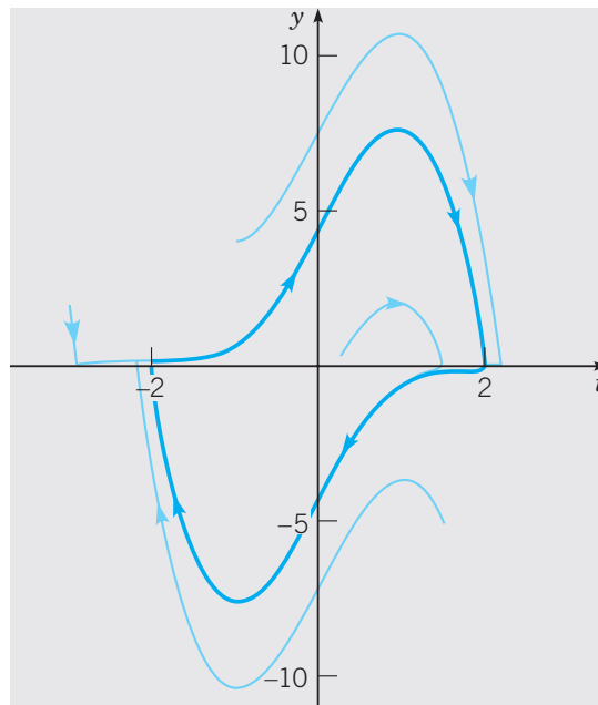
FIGURE 9.7.6 Trajectories of the van der Pol equation (17) for \mu = 5 .
