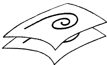
Fig. 85. A phase curve lies entirely on one level surface of an integral
